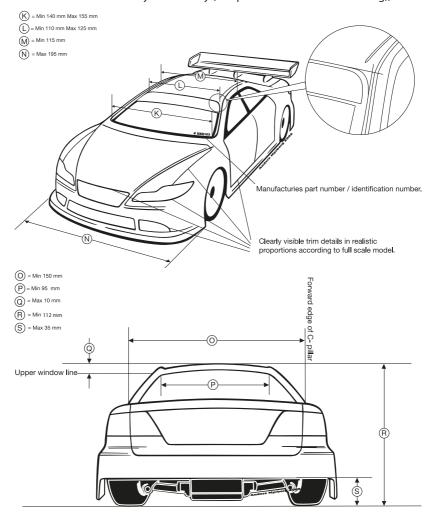
To assist competitors maintain consistent heights when using different wheels/ tyres, dimensions R and S will be measured with the chassis on a 15.0 mm block. Dimensions will be based on a 5 mm ground-clearance and will therefore be :- R = 122 mm, S = 45 mm.
