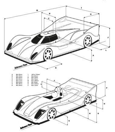
The body side forward of the side dam must have a radiused edge, no lips or upward extensions are acceptable
